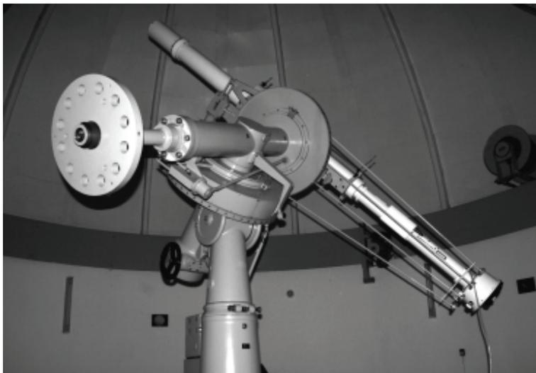
Figure 3. The new coronagraph of the Institute of astronomy assembled in Solar tower at NAO – Rozhen.
