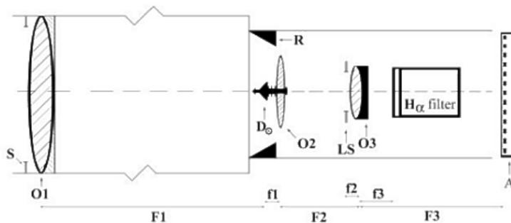
Figure 2. An optical scheme of the coronagraph.
