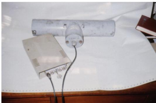
Figure 3. The prototype of the device for monitoring of the ELFs signals, consisting of ferrite antenna and ELF radio detector.
