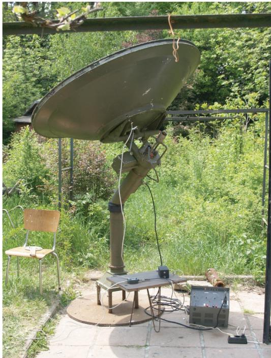
Figure 1. The prototype of the 1.5 m radiotelescope for monitoring of the X band solar flux, now equipped with commercial satellite detector.
