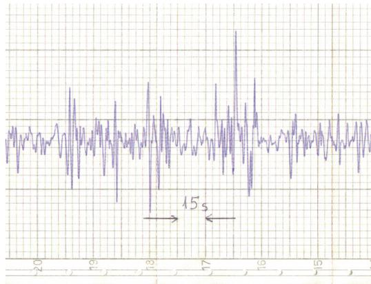
Figure 4. Flux registration of four ELF signal packets separated by 30–40 s, observed in the range 0.5–15 Hz with maximum sensitivity at about 2 Hz.
