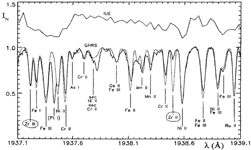
FIGURE 1 The ultraviolet (UV) spectrum of  $\chi$  Lupi obtained with the GHRs and with the IUE satellite (Leckrone et al., 1993), where the resolution of the spectrum obtained with the GHRs is 0.0023 nm and the maximal signal-to-noise ratio is 95 (Brandt et al., 1999): —, observed GHRs spectrum; ----, synthesised spectrum.
