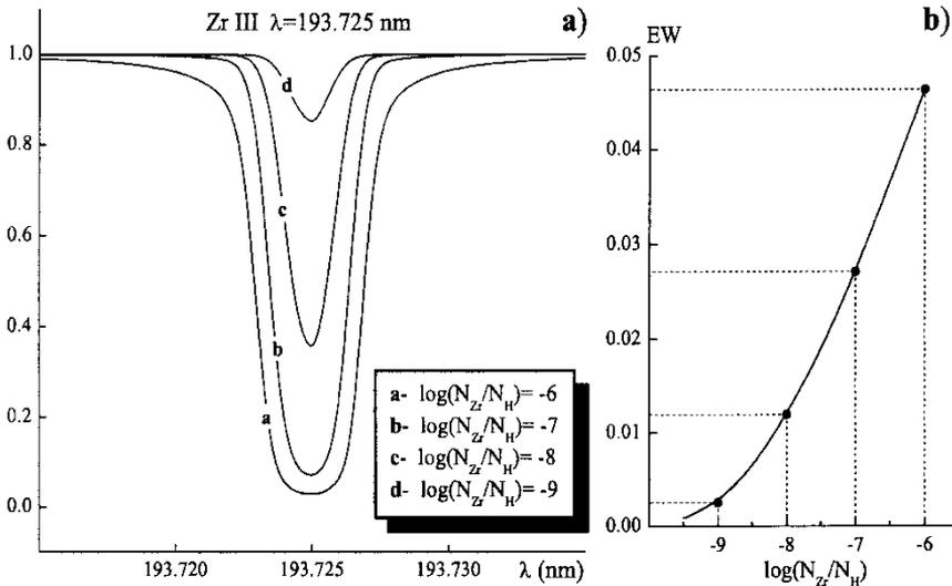
FIGURE 4 (a) The change in the Zr III  $4d^2 \ ^3P_1 - 4d5p \ ^3P_0^0$  ( $\lambda = 193.725$  nm) line profile due to the change in the zirconium abundance  $\log(N_{\text{Zr}}/N_{\text{H}})$  for the stellar atmosphere model with  $T_{\text{eff}} = 10,500$  K,  $\log g = 4.0$  and the turbulence velocity  $V_t = 0.0 \text{ km s}^{-1}$ . (b) The equivalent width as a function of the zirconium abundance.
