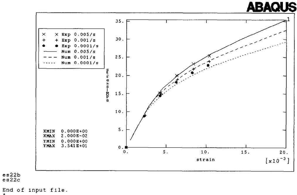
Fig. 2. The comparison of experimental response for samples cut at 32° from the machine direction with the predictions from the MRS model.
