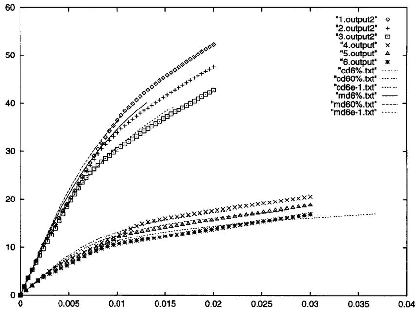
Fig. 3. The comparison of experimental machine direction and cross-direction stress–strain response with the predictions of the GUV model.
