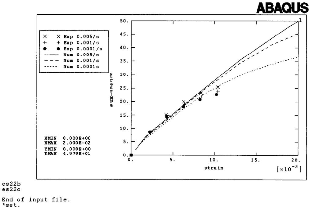
Fig. 4. The comparison of experimental response for samples cut at 32° from the machine direction with the predictions of the GUV model.
