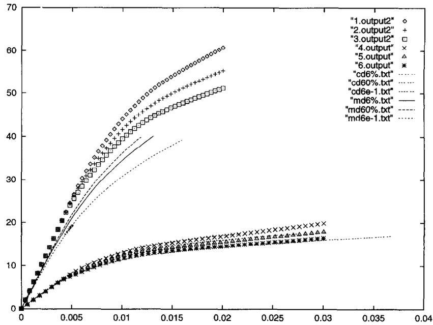
Fig. 1. The comparison of experimental machine direction and cross-direction stress–strain response with the predictions of the MRS model.
