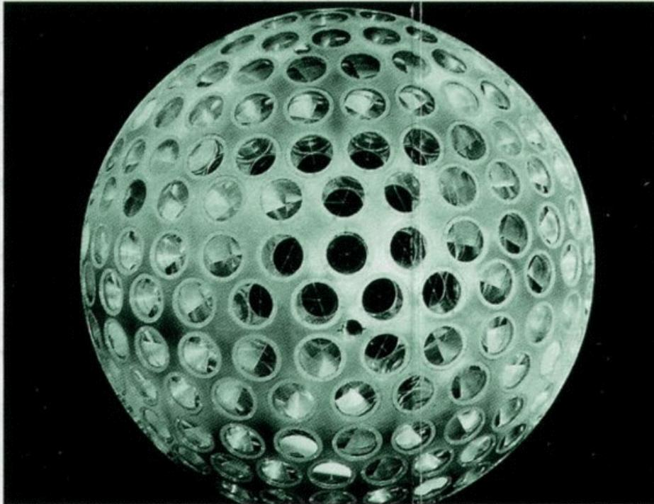
Lageos is the major SLR target used for IERS. It is a 60 cm diameter metallic sphere covered with retroreflectors, cruising at an altitude of 6000 km. It was launched in 1976 by NASA and will remain an excellent geodetic target for tens of thousands years.
