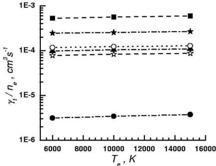
Fig. 1. The ratio of the total width to the electron density ( $n_e = 10^{14} \text{cm}^{-3}$ ) as a function of the electron temperature  $T_e$  for the studied Ar I lines (■ 522.1, \* 549.6, ○ 518.8, ▲ 603.2, \* 560.7, ● 696.6 nm)
