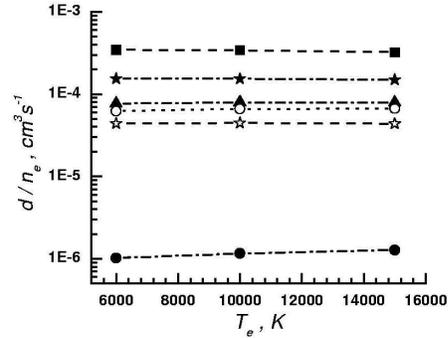
Fig. 2. The ratio of the shift to the electron density ( $n_e = 10^{14} \text{cm}^{-3}$ ) as a function of the electron temperature  $T_e$  for the studied Ar I lines (■ 522.1, \* 549.6, ▲ 518.8, ○ 603.2, \* 560.7, ● 696.6 nm)
